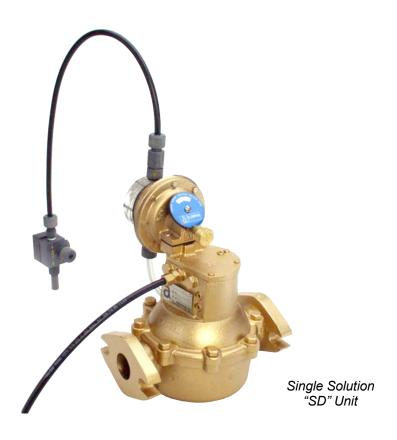
The S Series injector is the most reliable water powered proportional injector available. With over 50 years of proven service, no other product on the market comes close to matching the S Series' record of accuracy, dependability and value. Works with flows from 4 to 50 gallons per minute and ratios up to 1:160. Stronger and/or multiple solutions are available by adding an external manifold and pumpers.
