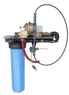
The DB Series offers an inexpensive way inject almost any liquid into a water line at an adjustable ratio. These pumps will inject one chemical up to a 1:100 ratio and 20 GPM. These models feature an adjustable feed ratio which makes fine tuning the injection ratio as easy as twisting a knob. Injectors can be turned down to 1/10th of their maximum feed ratio.
