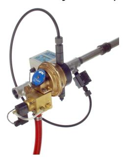
The DB Series offers an inexpensive way inject almost any liquid into a water line at an adjustable ratio. These pumps will inject one chemical up to a 1:100 ratio and 20 GPM. These models feature an adjustable feed ratio which makes fine tuning the injection ratio as easy as twisting a knob. Injectors can be turned down to 1/10th of their maximum feed ratio.
